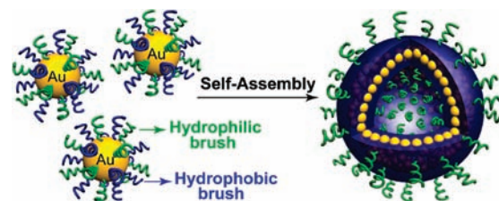
Figure 1. Schematic illustration of self-assembly of amphiphilic nanocrystals with mixed polymer brushes into vesicular structures.
